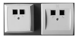
The VDSL modem shall be connected to the left located RJ11 jack of the NTP with an appropriate patch cord.
